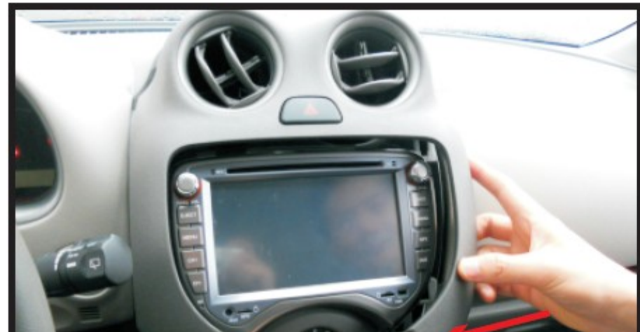
7. Install the housing of the air outlet and connect the wires. Be care of the buckles.
