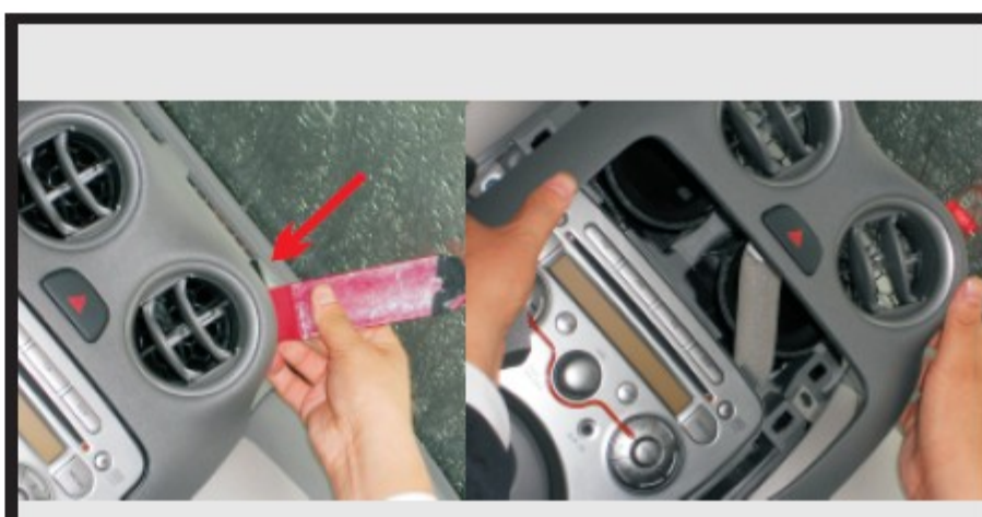
2. Pry the housing of the air outlet of air-conditioner, unplug the wires behind and remove it. Be care of the buckles.
