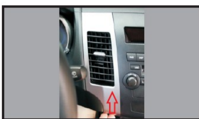
2. Put an upward force on the air conditioner frame and remove the outlet.
