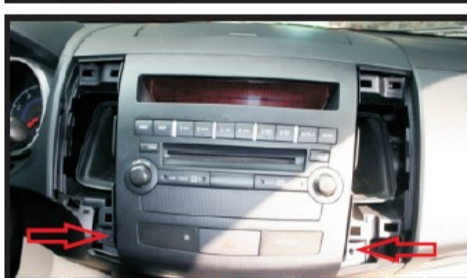
4. Pry the screws and the original board of head unit, and unplug the back wires of the head unit.
