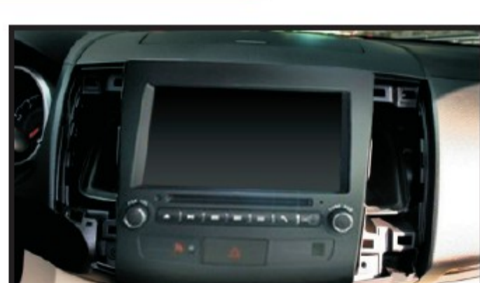
10. Plug the back cables of the head unit and put the USB cable to the glove box. Install our unit and fix the frame with screws.
