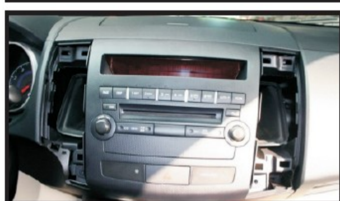
3. Take out the console behind the air conditioner outlet.
