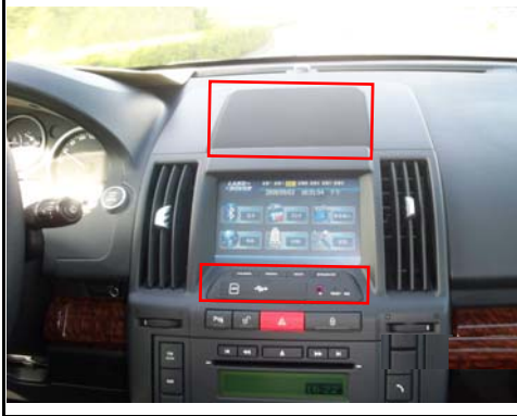
28、Close the unclenched cover of speaker to finish the assemble of monitor
