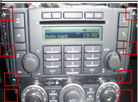
22、Firstly, Connect the wiring harness of original CD changer & air conditioner. Secondly, fix & screw the CD changer & air conditioner back.
