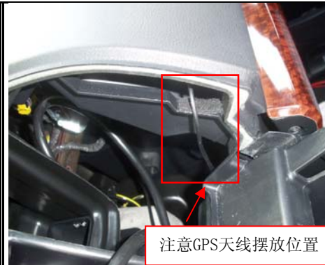
18、Take out the cover of air outlet of air conditioner; Put the antenna of GPS in the central control station Fix the grid cover of speaker back.
