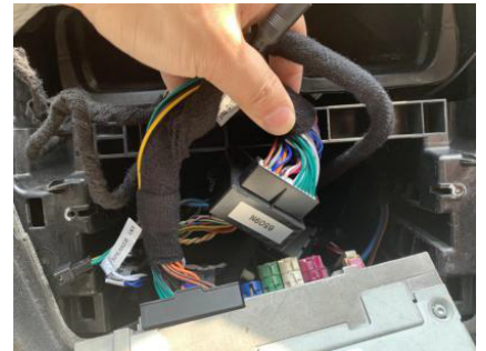
6. Pull out original harness and optical fiber, then plug it with Android power harness.
