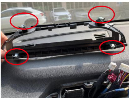
7. Remove the four Buckles on original stand base, and assemble it to Android stand base.
