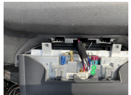
9. Plug well all the android cables. (Power/USB/4G/GPS)
