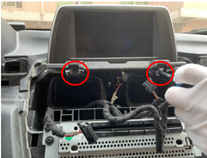
4. Remove two fixed screws of original monitor.
