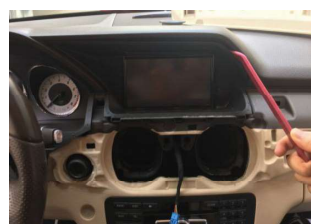
6. Pry loose and take out the frame of original monitor
