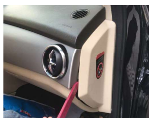
3. Pry out the side cover of glove box.
