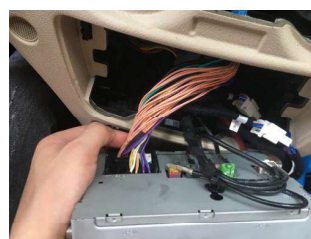
10. Remove the power harness from original host, and connect it to android harness.
