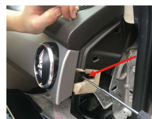
4. Remove the side fixing screws from air conditioning port
