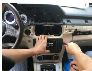
9. Pry out the original HOST
