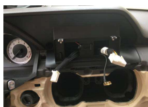
11. Assemble well the stand on Android monitor
