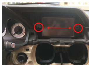
7. Remove the left and right fixing screws of the original monitor and take out the panel.
