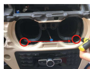
8. Loosen the left and right fixing screws of the original HOST
