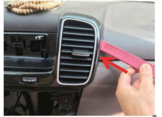
8. Pry out the air conditioner panel
