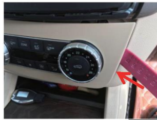
2. Pry the decorative frame of the air conditioner knob
