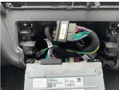
7. Pull out original harness and optical fiber, then plug it with Android power harness.
