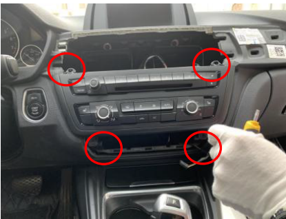
4. Remove four fixed screws of Panel.
