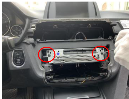
5. Remove two fixed screws of original HOST.
