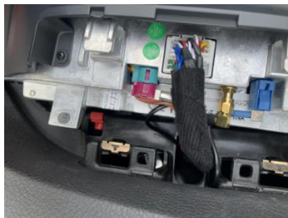
8. Plug well all the android cables. (Power/USB/4G/GPS)
