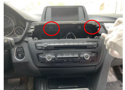
6. Remove two fixed screws of original monitor.
