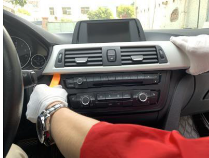
2. Take out the decorative sheet of air-conditioning.
