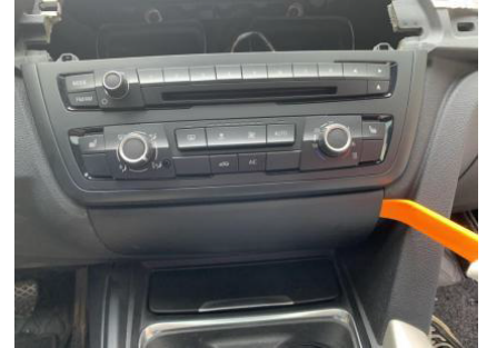
3. Pry loose and take out the panel of CD player.
