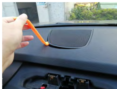
8. Pry loose the net and take out the center speaker.
