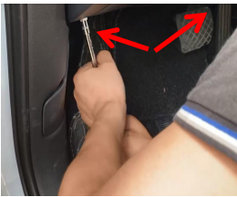
9.Remove the screws on both sides of the bottom of the main driving baffle
