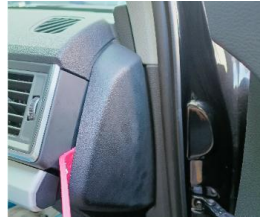
2. Pry out the right side baffle
