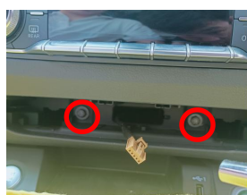
14. Unscrew the retaining screw
