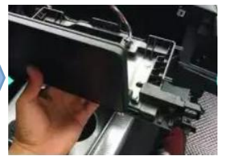
25.Remove the original display screen
