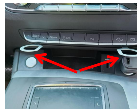
13. Remove the function board with a lock
