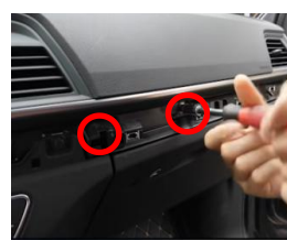
15. Unscrew the air conditioner air outlet 1
