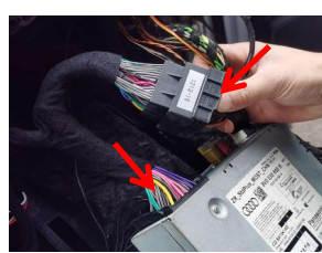
19. Transfer to our power line
