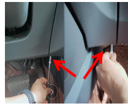
11. Remove the screws on the left and right sides of the bottom plate
