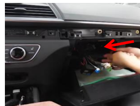
19. Unscrew the inside of the glove box
