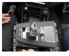
10. Pry out the central control gear cover
