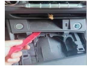
12. Remove ignition switch panel
