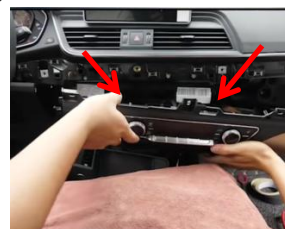
20. Remove the air conditioner control panel
