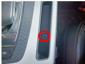
5. Unscrew the retaining screw
