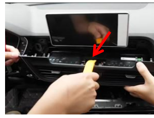
24.Remove the air conditioner air outlet panel 3
