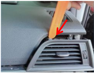
22.Remove the air conditioner air outlet panel 1
