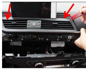
23.Remove the air conditioner air outlet panel 2
