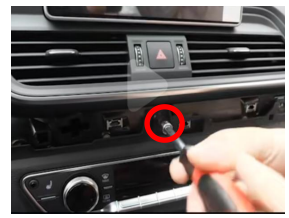
16. Unscrew the air conditioner air outlet 2
