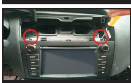
8. Tighten the two fixing screws.
