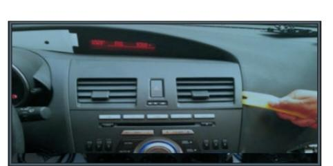
2. Pry the air outlet plate as shown in the picture with crow plate.
