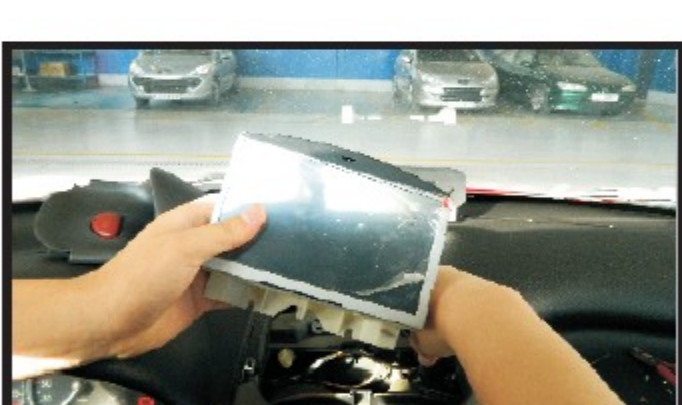
14. Connect all the cables with the corresponding harnesses of our display screen
