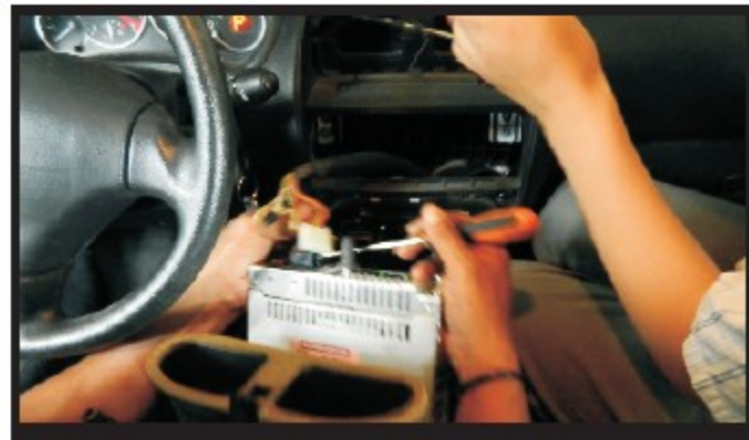
7. Take off the original control frame of the air conditioner.
