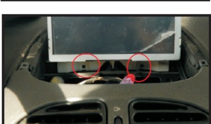
15. Fix our display screen with the screws, tighten
