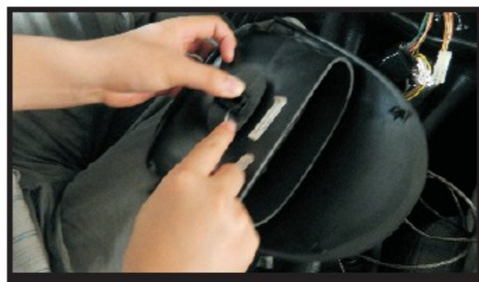
3. Take down the emergency button and small display screen from the frame carefully.
