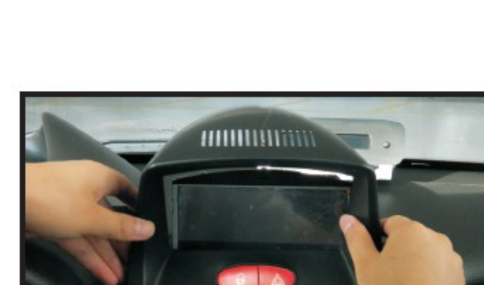
17. Connect the cable of emergency button and install the frame to the right place.
