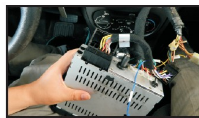
12. Connect all the cables with the corresponding harnesses of our DVD player
