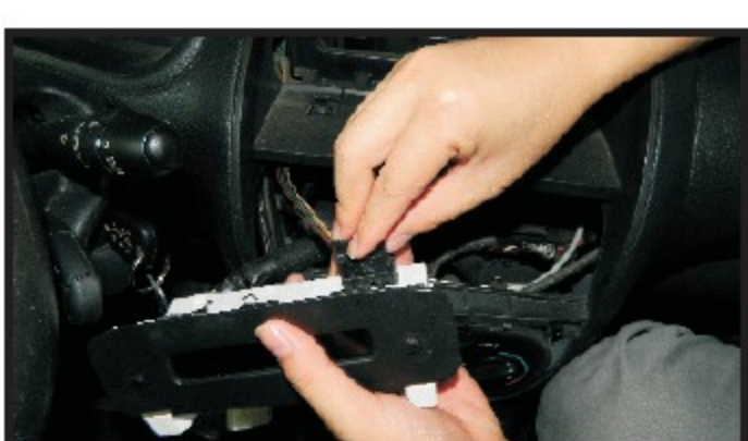
9. Connect the original small display screen with the cable
