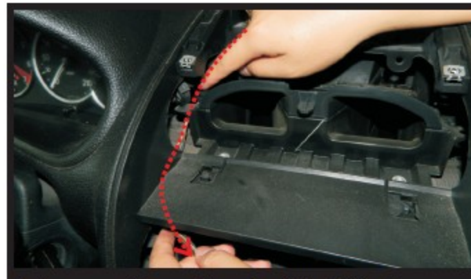
8. Arrange the cable of original display screen on the right place like the red dotted line.
